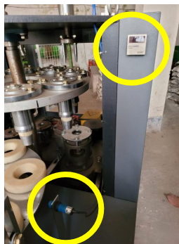
POINT D: COUNTER & SENSOR
